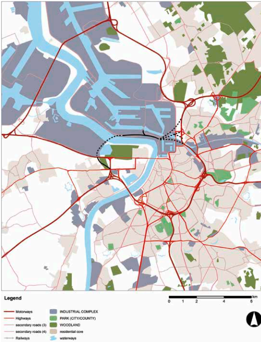
Figure 100 ABM Alternative variant 3, black large dots: viaduct, black small dots: tunnel. Source: based on AWV and Limehome fig. 2.3 p. 2.7 Overheidsstudie AWV Bestek/98C8, 1/03/2000 ( https://nl.wikipedia.org ).
